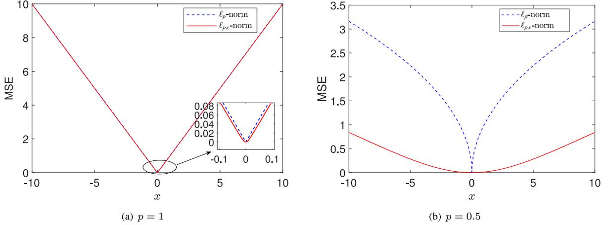
Fig. 2.  $\ell_{p,\epsilon}$ -norm and  $\ell_p$ -norm in one-dimensional case. Left:  $\epsilon = \sqrt{1-p} \times \max(x) + 10^{-2} = 10^{-2}$ . Right:  $\epsilon$  is calculated by  $\epsilon = \sqrt{1-p} \times \max(x) + 10^{-2} = \sqrt{0.5} \times 10 + 10^{-2} = 7.081$ .
